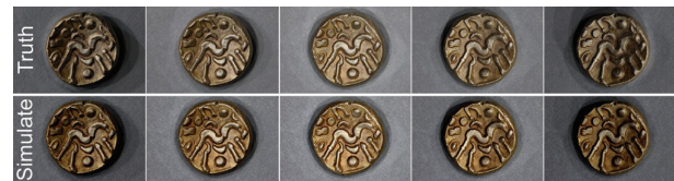
Fig. 13. To validate our design using an overlay across multiple lighting directions we simulate the effect of moving a light across a 90 degree arc of illumination angles. Five frames from the resulting sequence are shown here. The average RMS error across all frames is 5.0%, and nowhere does the error exceed 6.3%, remaining relatively consistent across the full range of lighting angles.
